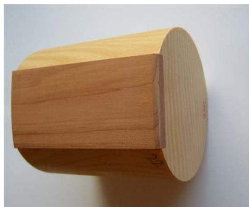
**Position 2 block low** – two strips of adhesive tape are on either side of the top of the block, on the air exit side.
